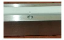
2. Place thermocouple through hole in jaw:
