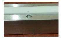
2. Place thermocouple through hole in jaw:
